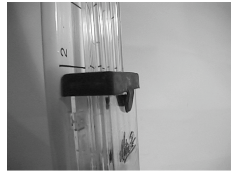
Vent in Closed Position
