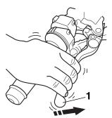
11.After the pulsating action has stopped in the brake lever, it is generated in the brake pedal "1" 0.5 second later and continues for approximately 2 seconds.
