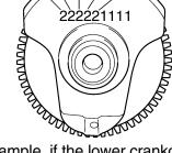
For example, if the lower crankcase  $J_1$  and crankshaft web  $J_1$  numbers are 6 and 2 respectively, then the bearing size for  $J_1$  is:
